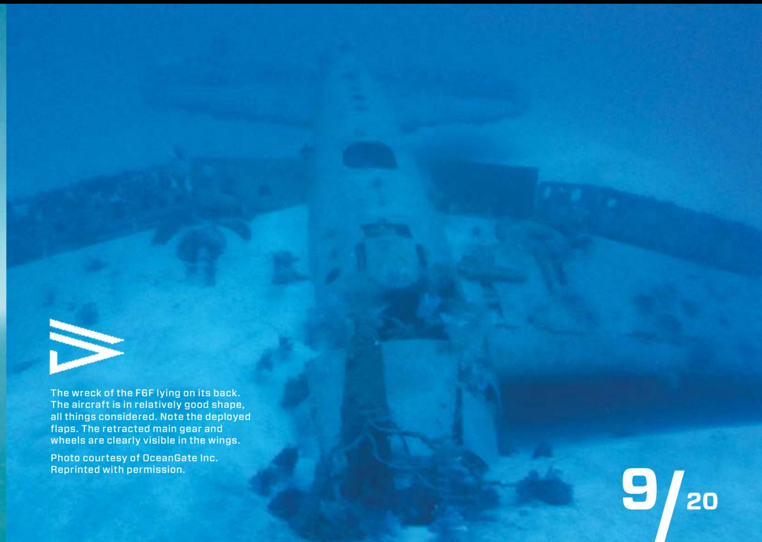
The wreck of the F6F lying on its back. The aircraft is in relatively good shape, all things considered. Note the deployed flaps. The retracted main gear and wheels are clearly visible in the wings.
